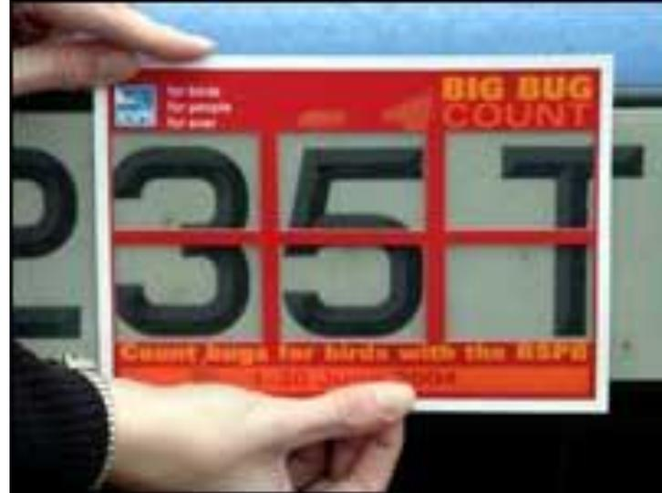
The ‚splatometer‘ is fixed to vehicle number plates.
